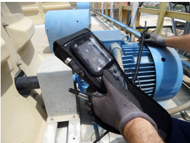
Figure 1. Manual inspection of equipment using piezo sensors and a handheld logger.
