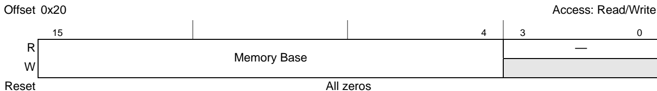
Figure 17-77. PCI Express Memory Base Register
