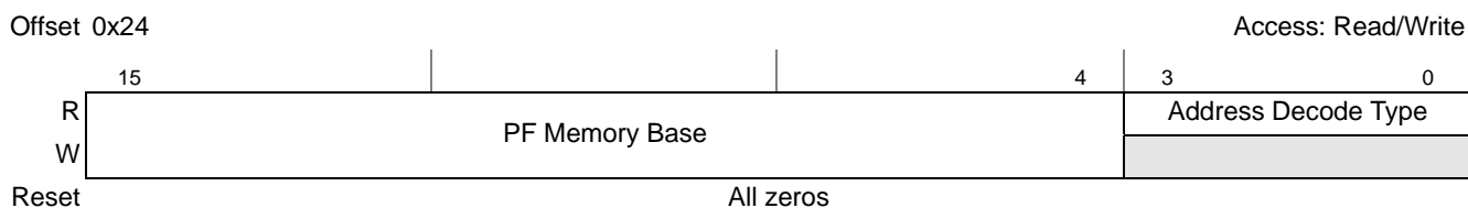
Figure 17-79. PCI Express Prefetchable Memory Base Register
