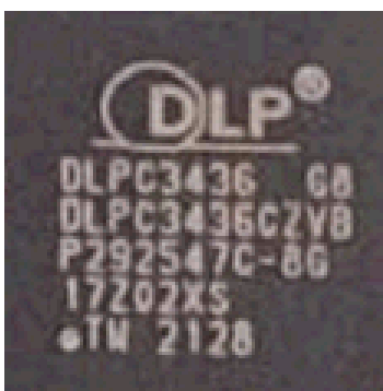
After Change – 4 th row "17Z02XS" shows standard TI assembly Lot Trace Code
